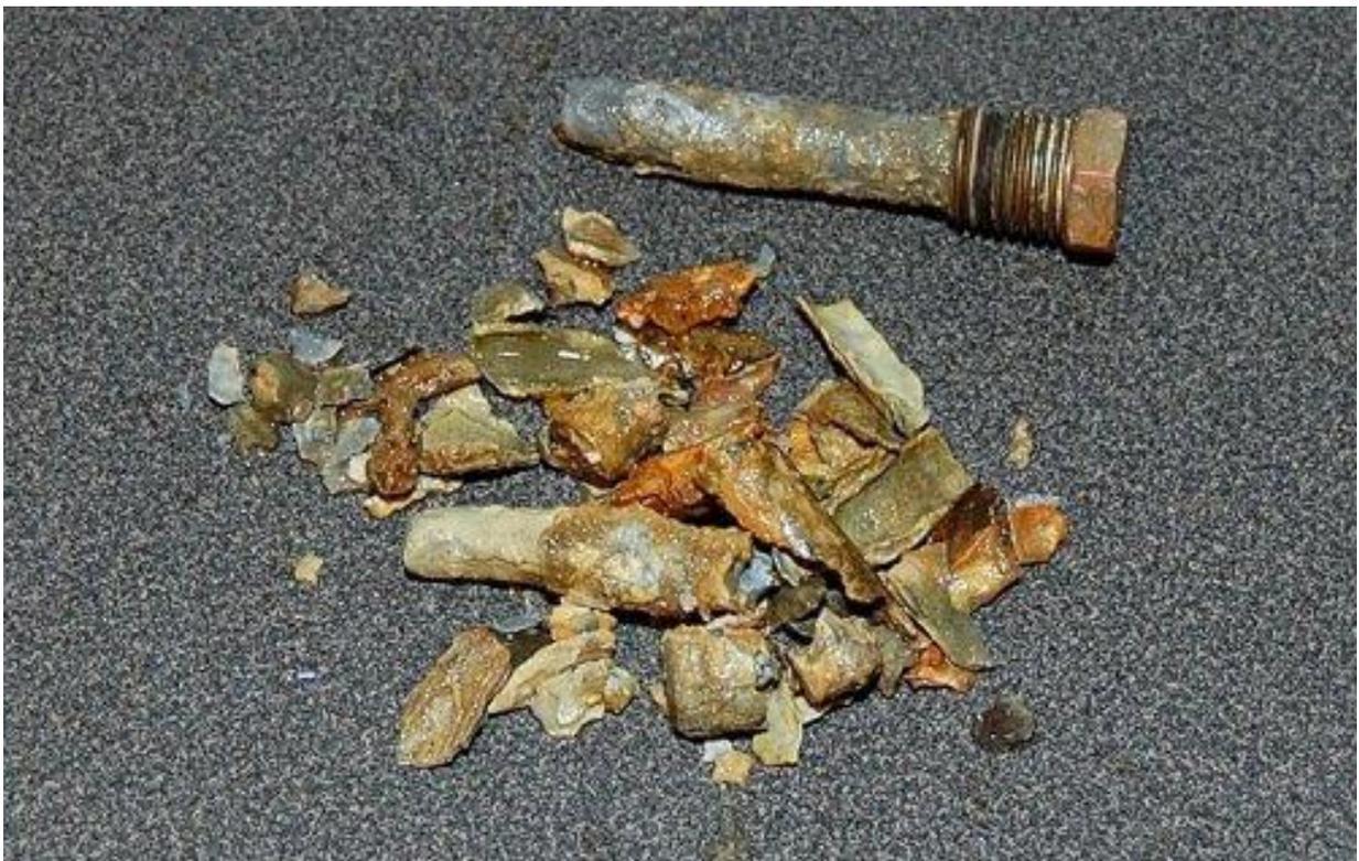
Zinc anodes in the engine's cooling system wear out like any other anode. Forgetting to replace them can lead to corrosion, ruining expensive components.
