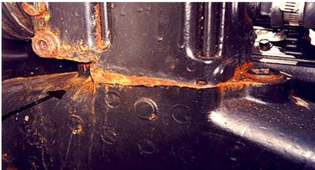
A quick check of the outside of your risers can tell you a lot about the inside. If you can see rust streaks, chances are there is corrosion inside as well. A corroded riser can allow water inside the engine, destroying it.
