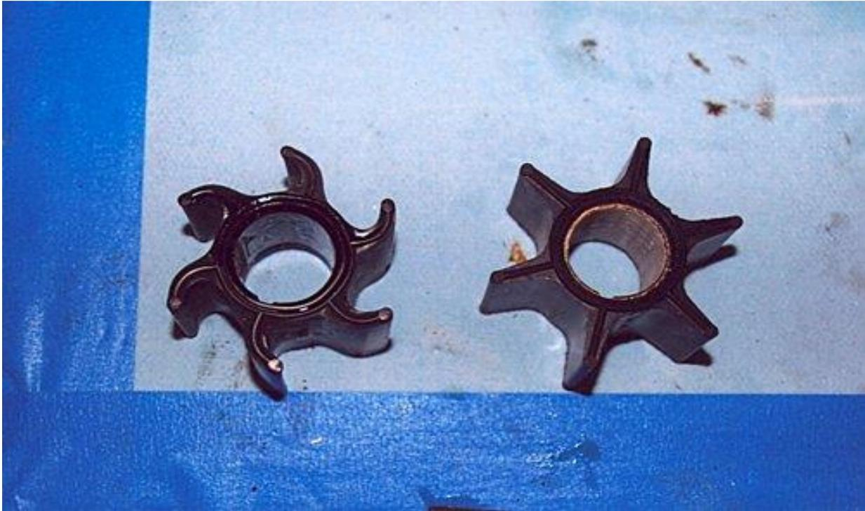
The impeller on the left is worn out; the vanes could break off and get stuck in your engine's cooling system, causing overheating. Now is the time to replace it if you haven't done it in a couple of years.
