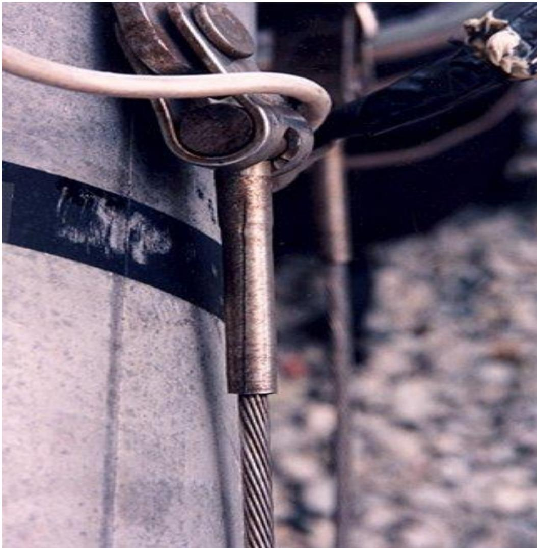
A few minutes checking swage fittings can save your rig. Look for bulging or cracks like this that signal corrosion. Replace any suspect fittings immediately.
